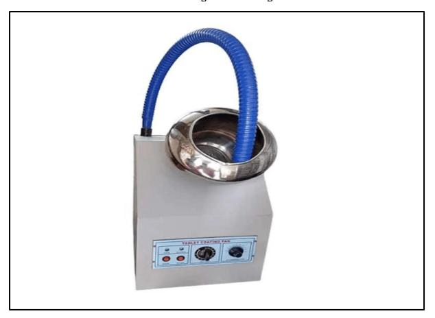
A tablet coating pan is a device used in the pharmaceutical industry to apply a thin, uniform coating layer onto tablets. This coating can serve various purposes, such as improving appearance, taste masking, protecting the active ingredient, or controlling drug release. Here's a brief overview:
