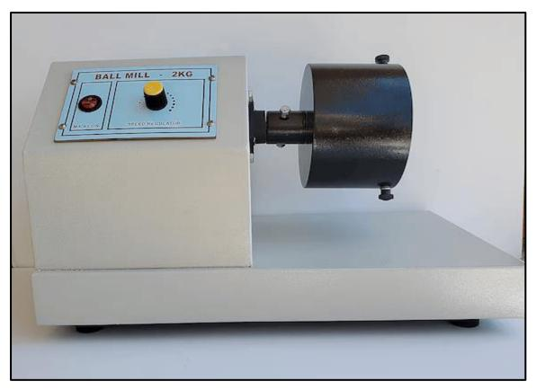
A Ball Mill is a grinding device used to crush and blend materials for various industries, including pharmaceuticals, mining, cement, and chemicals. It works by rotating a cylindrical chamber filled with grinding media (balls) to reduce material size through impact and friction.
