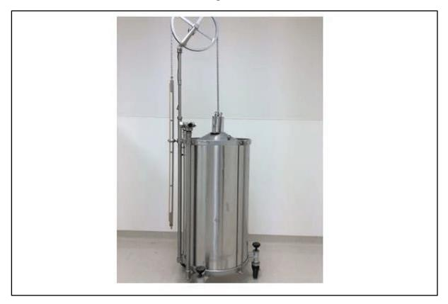
Hutchinson's Spirometer is a medical device used to measure lung capacity and respiratory volumes. It consists of a water-filled chamber with an inverted bell that rises and falls as a person breathes into it. The movement of the bell is recorded to determine vital capacity (VC) and other lung parameters. It is widely used in pulmonary function tests, respiratory research, and medical diagnostics.Modern versions include digital spirometers with electronic sensors for more precise measurements.
