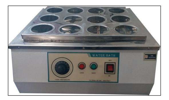
A **rectangular water bath** is a laboratory device used to heat or maintain samples at a constant temperature in a water-filled chamber. It is characterized by its rectangular shape, which provides a larger surface area for holding multiple samples simultaneously. Key features and applications include:
