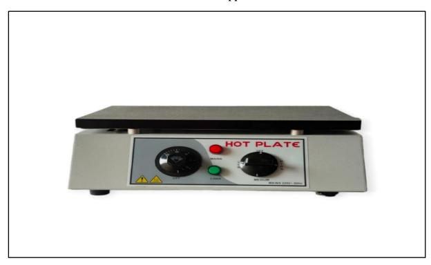
A **Hot Plate Apparatus** is a laboratory device used for heating substances evenly. It consists of a flat, heated surface (usually made of ceramic or metal) and is powered by electricity. Some hot plates come with a **temperature control knob**, **magnetic stirrer**, and **digital display** for precise heating.
