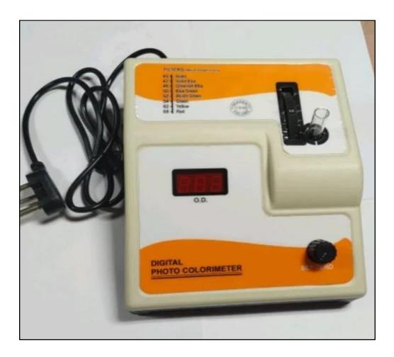
A **digital photo colorimeter** is an analytical instrument used to measure the concentration of a substance in a solution based on its color intensity. It works by passing light through a sample and measuring the absorbance of specific wavelengths of light. Key features and applications include:
